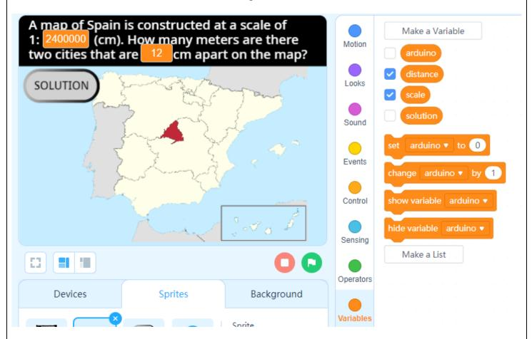
In addition, we will create the "Solution" variable, which will be the one that calculates the solution to the problem, and the "Arduino" variable, which will be in charge of sending to the Arduino board when and that the corresponding LED lights up.
