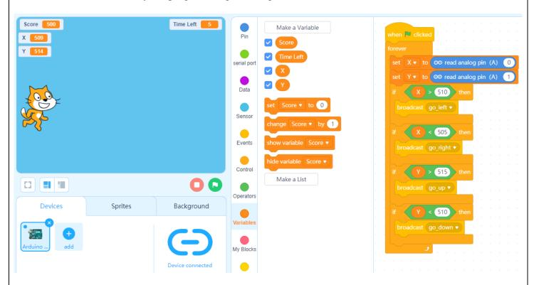
4. Next, we proceed to program the chronometer, which will count down. Really, the important thing is to start the variable "Time Left" in the seconds that we want the chronometer to have. In this case, it will be 30 seconds. Also, we indicate that the variables "Score" and "Time Left" are shown in the game so that the user knows his score and the time he has left to finish capturing the mice:
